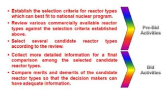
Fig.4. Five (5) steps of reactor technology selection
